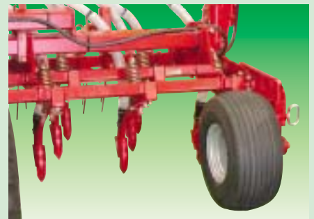
Floating frame system with slot A wheel (18X8.50-8 size) is available for controlling the work depth of the floating side frames with pin adjustment.
