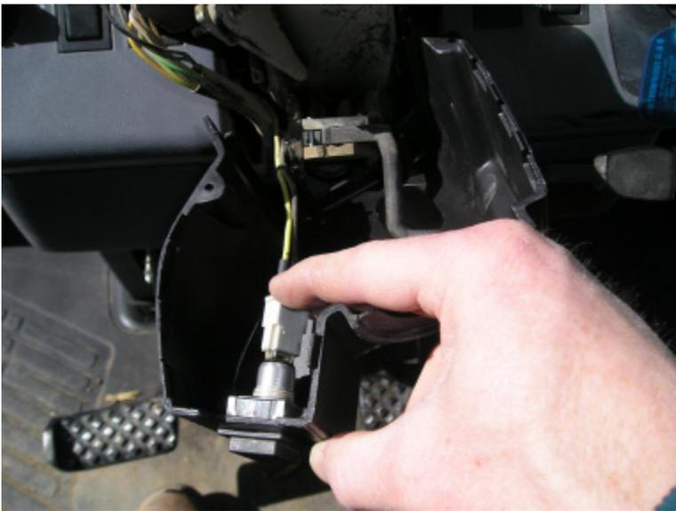
4. Reinstall the two lower screws in the plastic housings.
