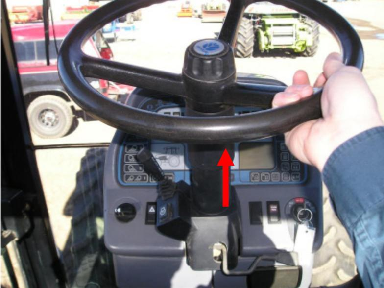
3. Remove the top two screws from the plastic housings covering the steering column.
