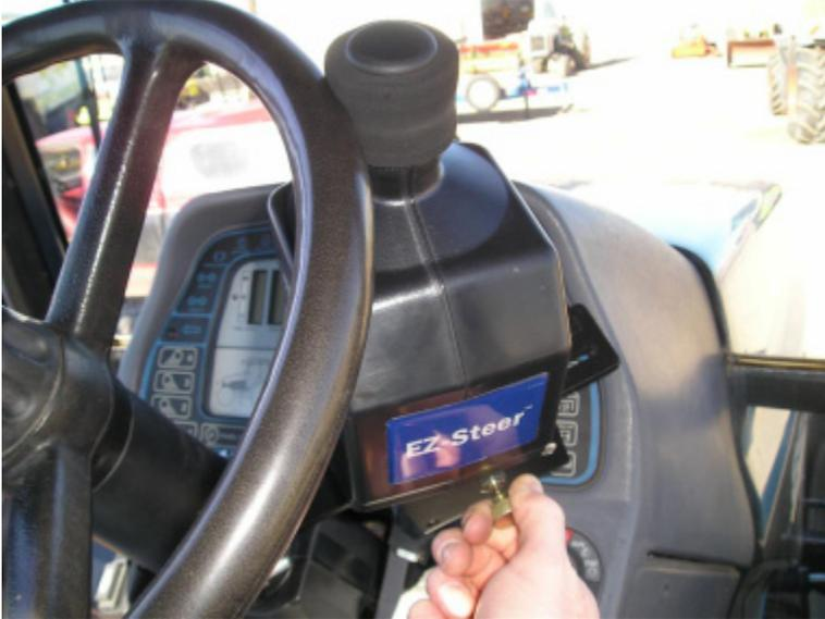
6. Make sure the center of the motor drive wheel is aligned with the center of the steering wheel outer ring.
