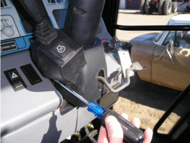
5. Remove the two-prong connector from the ether switch.
