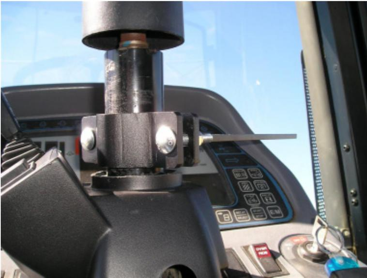
2. Squeeze the bracket clamps together. Use a ½ gear ratchet combination wrench to turn the nuts down against the clamp.
