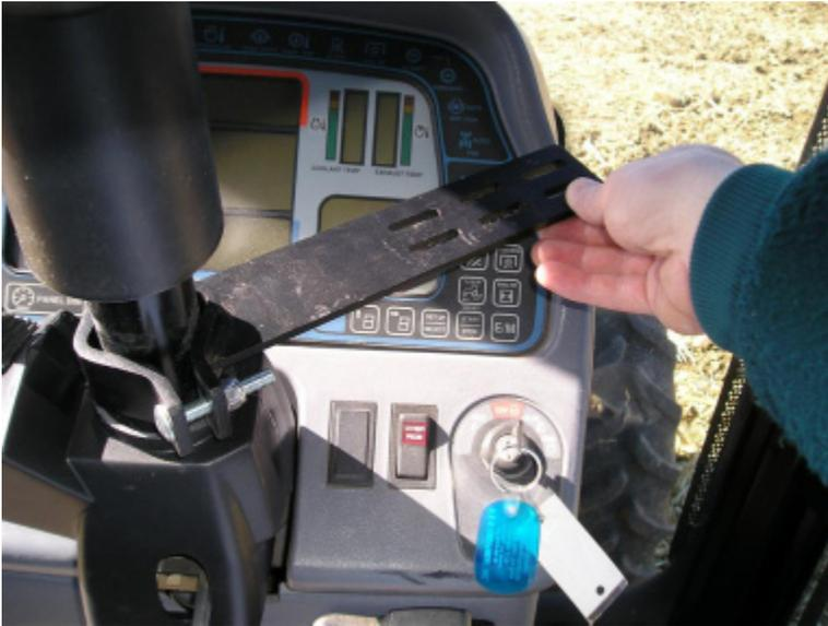
4. Tighten the bracket bolts to 4.1 Nm (3 ft-lbs) torque Use a ½ inch deep socket.
