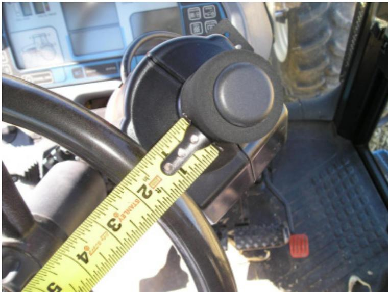
5. Pull the motor release knob. The motor will spring against the steering wheel.
