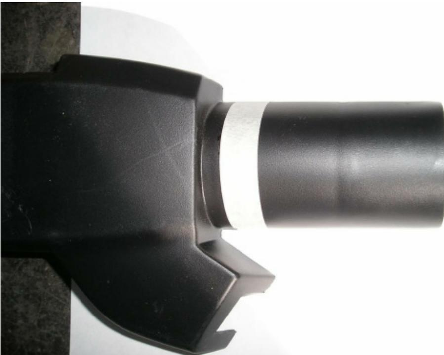
4. Set Dremel tool to 500 RPM and cut slowly. Follow the edge of the masking tape. Use the #561 cutting bit to cut the plastic and then the #470 sanding band to smooth the cut edge.
