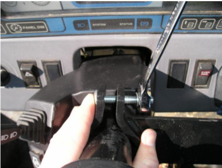
3. Rotate the bracket slotted arm to a 2 o'clock position. Ensure that the end of the bracket will not contact the dash.
