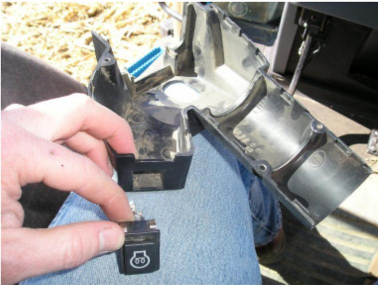
8. Tilt the steering column fully down and remove the upper housing.
