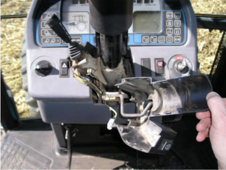
7. Remove the ether switch from the lower housing.
