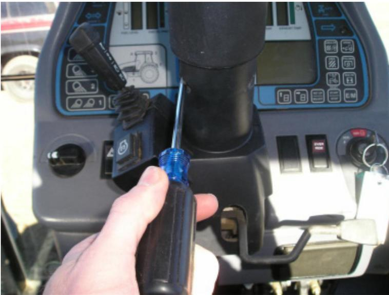
4. Remove the bottom two screws from the plastic housings covering the steering column.
